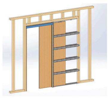
Once the door is operating correctly, cut Top Jamb to fit opening (ensure the cut end is located into the Door Stop Jamb)
