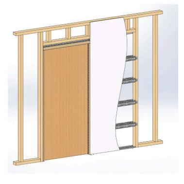
Door must be in closed position before plasterboard is fixed to ensure no damage when drilling holes
