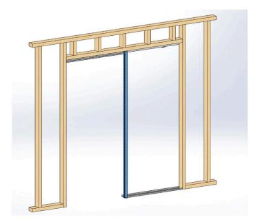
Insert Frame Uprights. Locate Frame Uprights into notches in the Frame Top Hat and the Bottom Channel.
